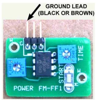
(Note that the **bottom** quadrants of both pots are blackened, to aid in visually detecting the fully counter-clockwise position as well as the degree of rotation.)
